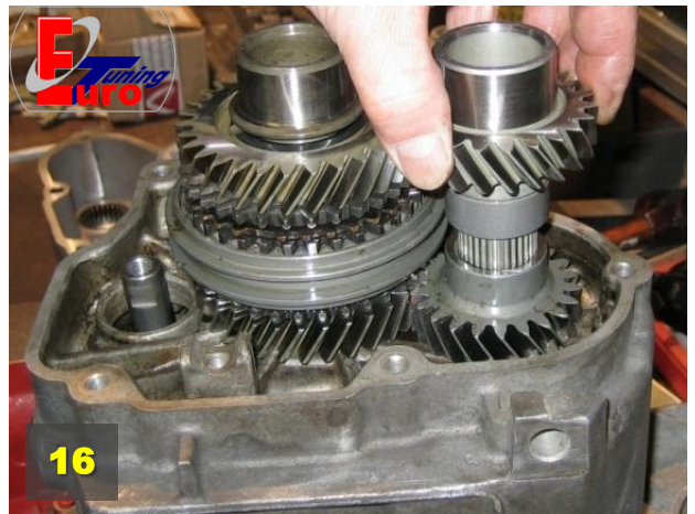
Fit driven wheel of 5th gear to splines of driven wheel of 6th gear
