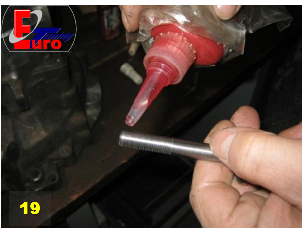
Fix bolts M10x1 with glue (red) Properly degrease the shaft thread and the bolt before gluing !
