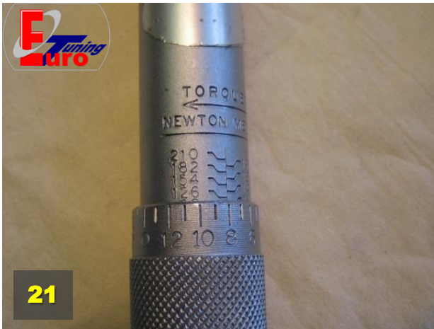
Tighten bolts M10x1 up to 120 Nm
