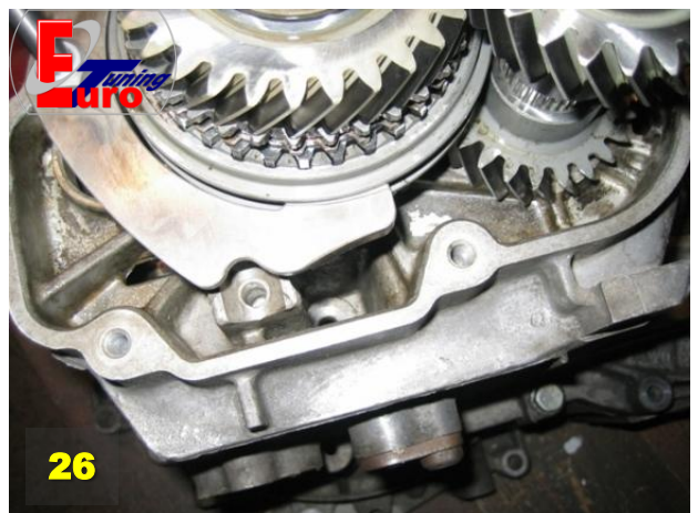
Apply securing glue (blue) to the end bolt thread and connect selector fork with selector rail by extender shift rail
