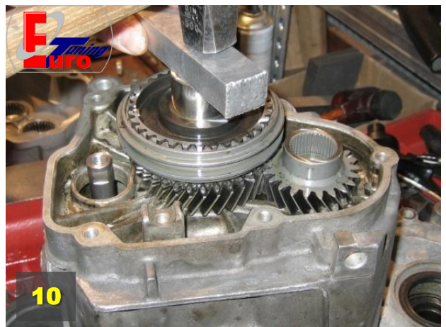
Move the synchronizing hub up to the stop (knocking over aluminium piece)
