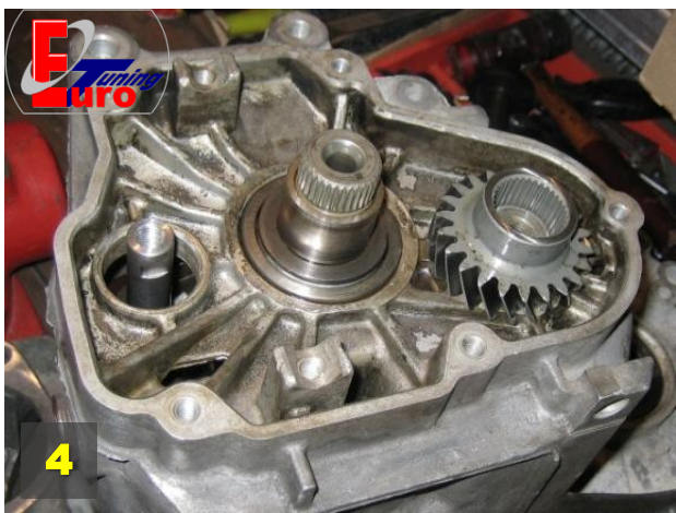
Fit the driven wheel of the 6th gear (knocking over aluminium piece)
