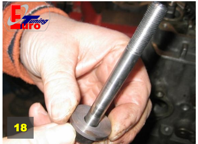
Fit flexible washers to shaft bolts (washer curve directed towards bolt head)
