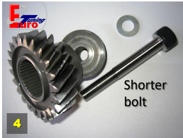
No knocking over aluminium piece, but tighten with a bolt and a mounting tool (100 Nm)
