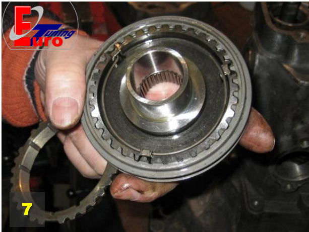
Complete synchronizing hub: core, dog gear, 3x locking latches, 2x spring
