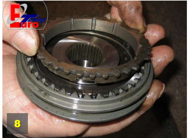
Fit the lower synchronizer ring (connect with the locking latches)
