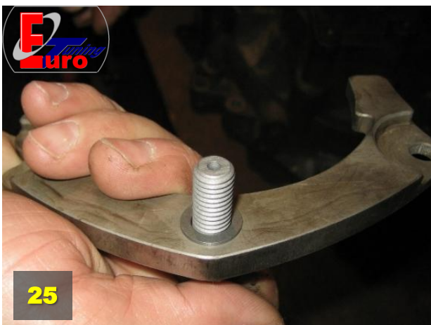
Adjust the centre position using ground washers between shift rail and selector fork
