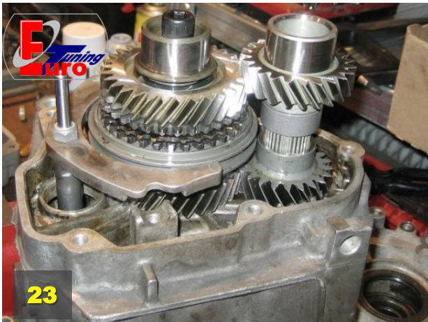
Connect selector fork with gear shift rail using the end bolt
