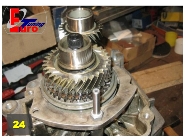
Check, whether the dog gear has the same distance to both ends of the synchronizing hub (top and bottom) in idle speed
