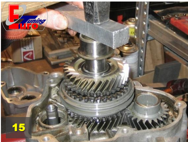
Move the idler spindle needle cage up to the stop (knocking over aluminium piece)
