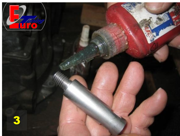
Screw on the gear shift rail extender, secure with glue (blue)
