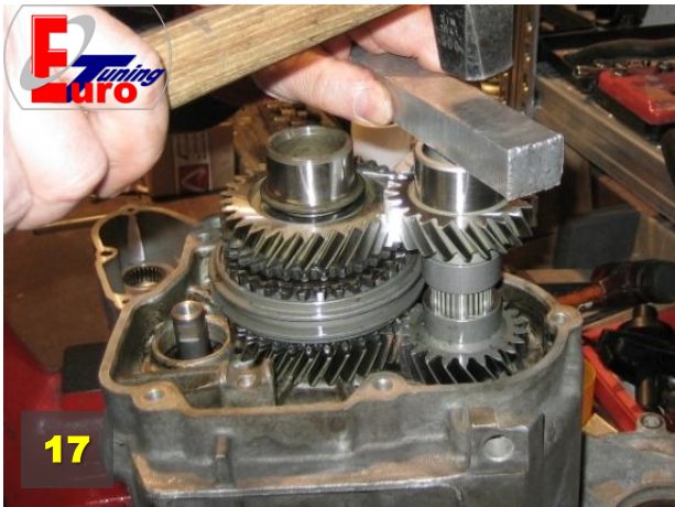
Move the wheel of 5th gear up to the splines - up to the stop (knocking over aluminium piece)
