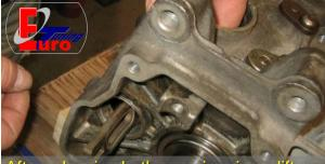
After releasing both securing rings, lift the shift rail, push it out of the gearbox through the hole at the shafts at the end of the gearboxs
