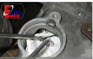
Then take a long tool with a magnet and take the securing ring under it and the washer out of the gearbox.
