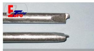
First modify a long screw-driver to make it able to loosen the securing sheet metal rings.
