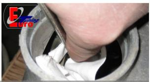
Install a cloth around the bolt, from which you loosen the securing ring using a long screwdriver to prevent it from falling down and hold it additionally with your finger when levering it out.
